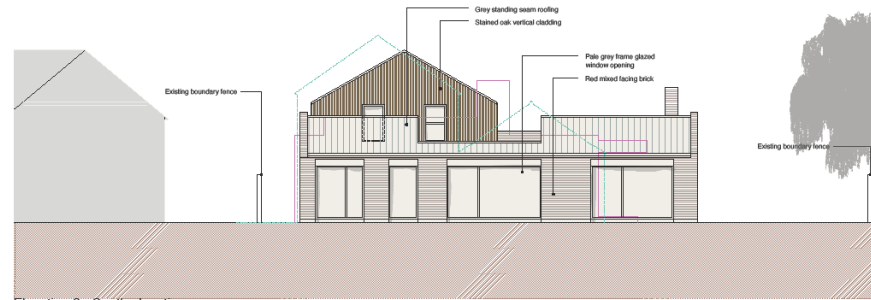
Elevation 2 - South elevation
